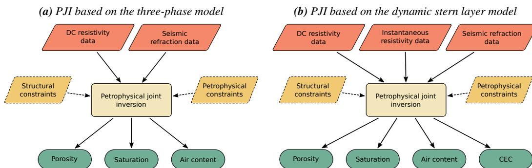
**Figure 1** Schematic illustration of the petrophysical joint inversion (PJI) schemes used in this study. (a) PJI of single frequency resistivities and seismic traveltimes to solve for porosity  $\Phi$ , saturation  $\Theta_w$ , and air content. (b) To take into account the surface conductivity, DC and instantaneous resistivity data have to be considered in the PJI.
