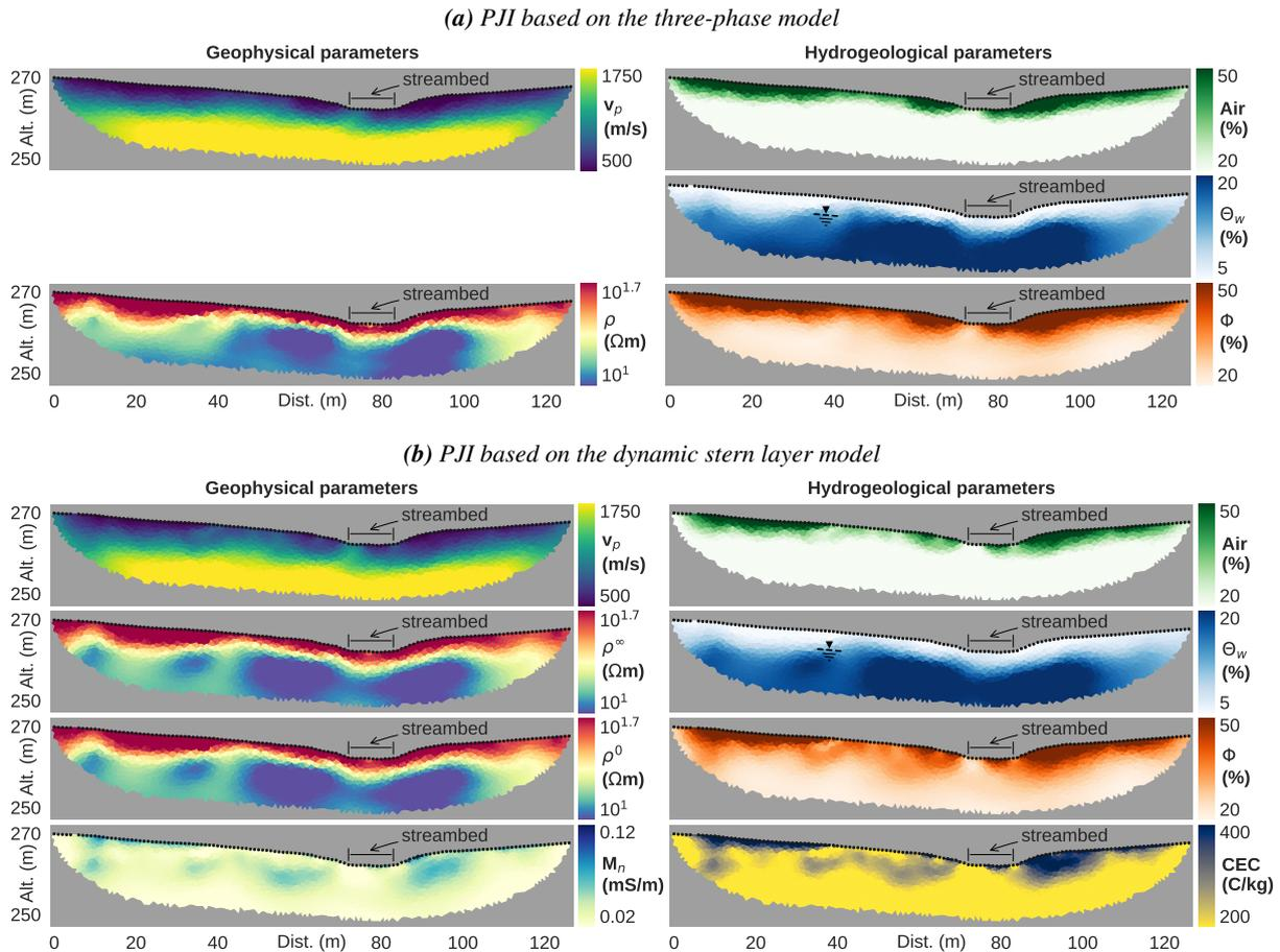
**Figure 2** Subsurface models resolved through the proposed PJI schemes. The black dots indicate the sensor/shot positions. The groundwater level observed in a borehole nearby is indicated in the resolved saturation model. (a) Subsurface air content, saturation and porosity. (b) Estimation of both  $\rho^\infty$  and  $\rho^0$  permits the computation of the normalized chargeability  $M_n$ . Additionally, the CEC is obtained through the application of this PJI scheme.
