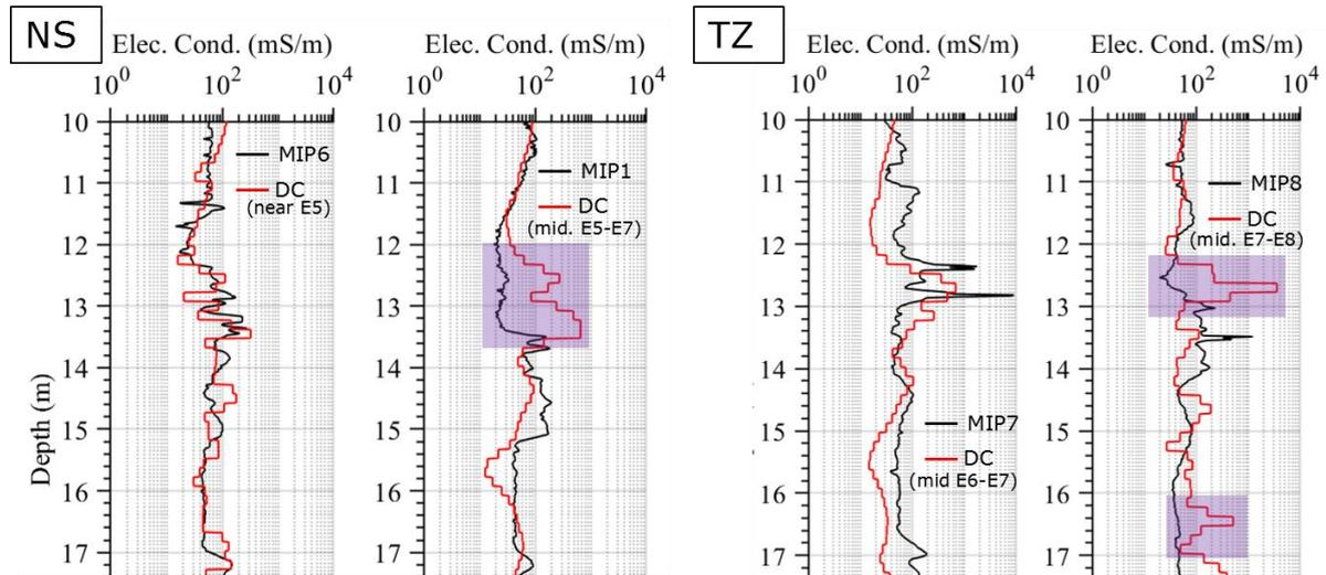
**Figure 2.** Comparison of “true” electrical conductivity measured by induction logs (MIP1, MIP6, MIP7 and MIP8, see location in Fig. 1) with inverted conductivity from cross-borehole ERT at Inj#2+20 days in Farum. The depth range 10-20 m corresponds to elevation range 19-29 m.
