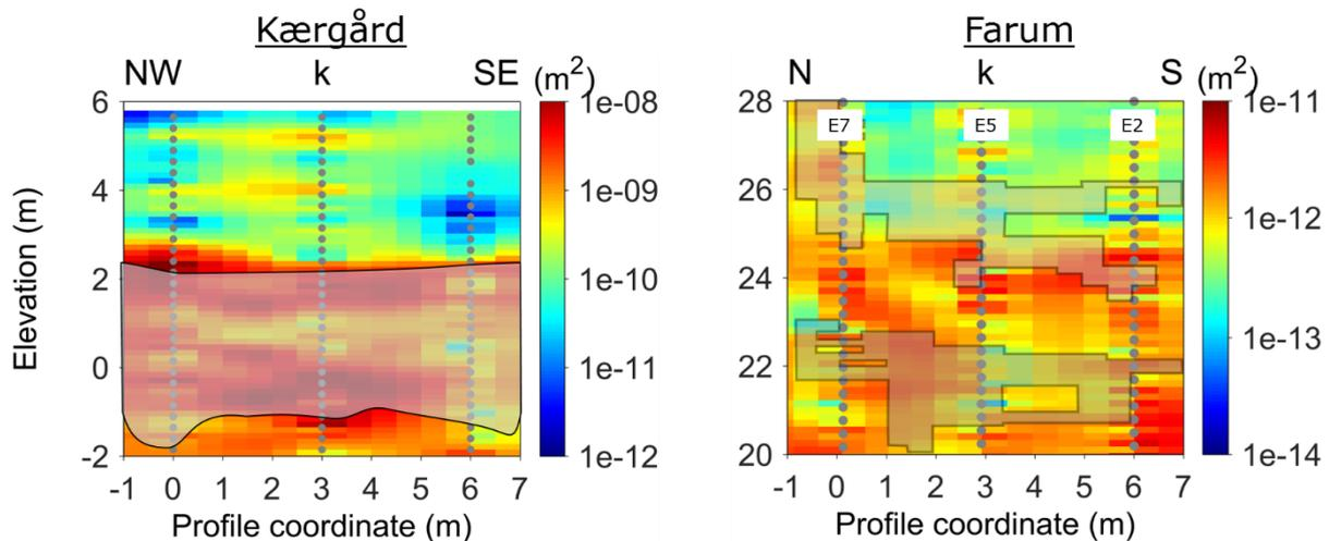
**Figure 3.** Permeability models obtained from cross-borehole DCIP inversion at Kærgård (left, published by Bording et al., 2021) and Farum (right). Note the different colour scales. The shaded grey zone indicates the distribution of the low-resistivity anomaly (all cells with a resistivity ratio lower than 0.3) along the profile at +1 day for Kærgård and +270 days for Farum. Electrodes are indicated by grey filled circles.
