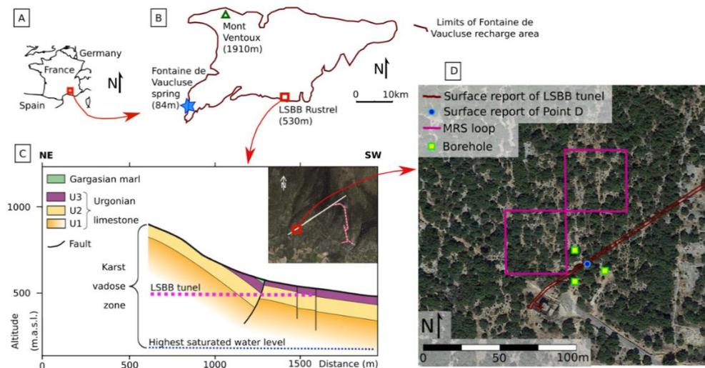
**Figure 1** Location of (A) test site in France; (B) in the Fontaine de Vaucluse karst hydrosystem; (C) schematic cross-section across LSBB; (D) overview of the respective locations of the LSBB tunnel, the three boreholes and the SNMR loop [Mazzilli et al., 2020, modified]
