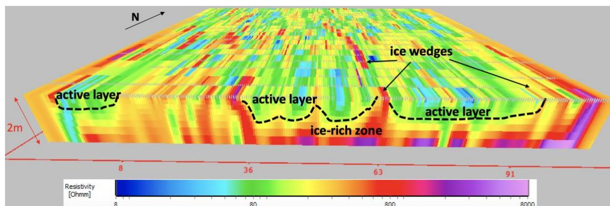
**Figure 4** The shallow 3D resistivity grid (100 m X 100 m X 2 m) seen from the top: it images the active (conductive) layer and ice wedges (long resistive ridges) characteristic of Adventdalen permafrost.
