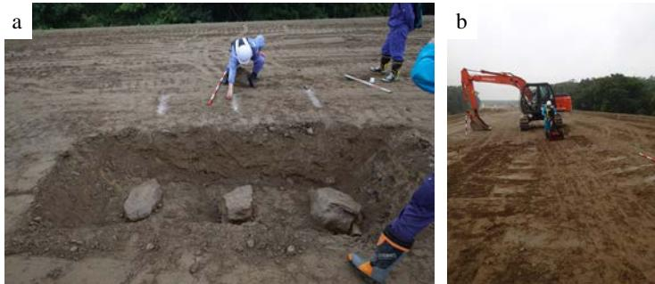
Figure 1: Photographs of the field experiment. Three different sizes of boulders were set in a pit (**a**). Then we covered the boulders with embankment materials. GPR survey was conducted (**b**).
