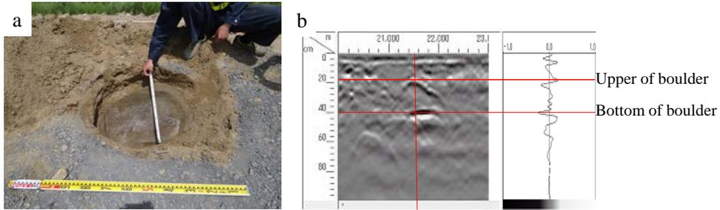
Figure 3: An unearthed boulder (a) and its GPR profile (b). A boulder was found at 15 cm in depth. As shown in b, the upper reflection waves generated by the buried boulder was positive polarities, and the bottom reflection waves generated by buried boulder were negative polarities.
