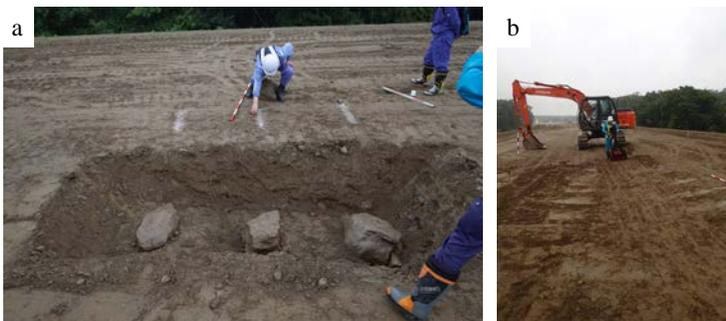
Figure 1: Photographs of the field experiment. Three different sizes of boulders were set in a pit (a). Then we covered the boulders with embankment materials. GPR survey was conducted (b).
