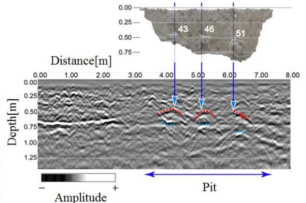
Figure 2: An example of GPR profile. Red dotted line indicate the reflection waves generated by the upper parts of boulders. Blue ones indicate the reflection waves generated by the bottom parts of boulders.
