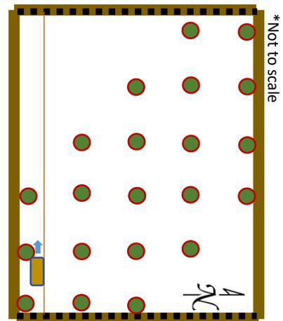
**Figure 2:** Diagram showing the top-down view of our frame. Green circles indicate plants. The dark yellow box is the instrument and the orange line is a guide string. Black dots represent guide holes drilled on 5 cm centers.
