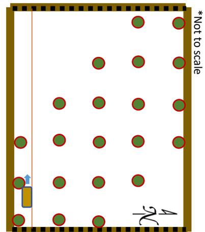
**Figure 2:** Diagram showing the top-down view of our frame. Green circles indicate plants. The dark yellow box is the instrument and the orange line is a guide string. Black dots represent guide holes drilled on 5 cm centers.
