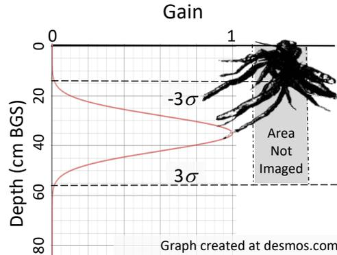
**Figure 4:** Gain (depth-determined) applied to the GPR data to accentuate data below 10cm BGS. Image of cassava roots scaled to size are shown next to the chart.
