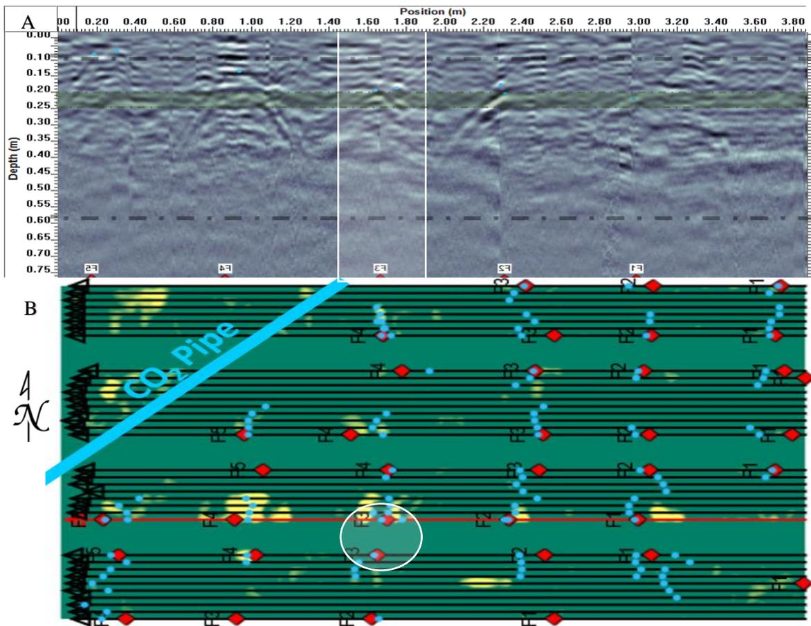
**Figure 5:** Partially processed GPR data that was gathered immediately prior to the third and final harvest of the season. A. a vertical section: B. a depth slice.
