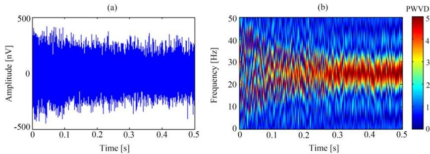
**Figure 1.** The noisy MRS oscillating signal and the time frequency distribution of its analytic signal. (a) Simulated MRS oscillating signal which embedded in random noise; (b) PWVD of the analytic signal.
