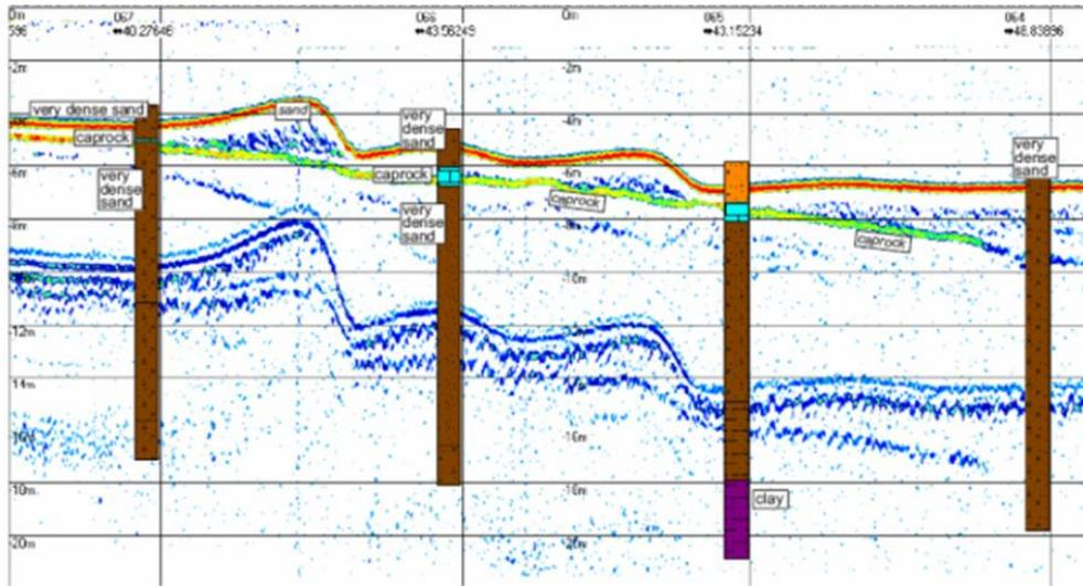
**Fig.4: Combined Interpretation Borehole and Acoustic Data**
