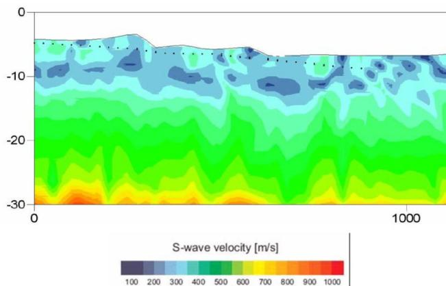
**Fig. 8: Combined Acoustic & MASW 2D profile**
