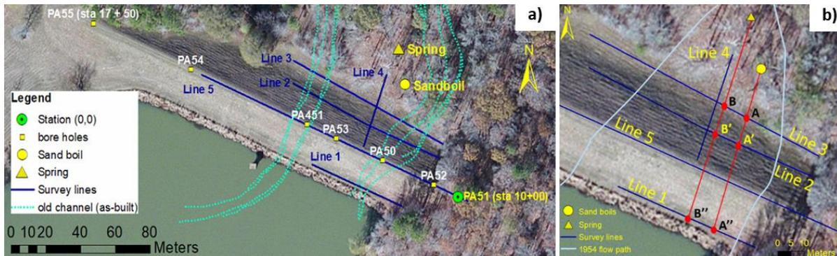
**Figure 3:** a) Present-day Google Earth images showing the location of survey lines, the position of the boreholes and other points of interest. b) Location of the interpretation points A, A', A''; B, B', B'', which represents the intersections points of two straight lines (in red) one starting from the spring and the other starting from the sand boil, used as reference locations in the interpretation of the geophysical data.
