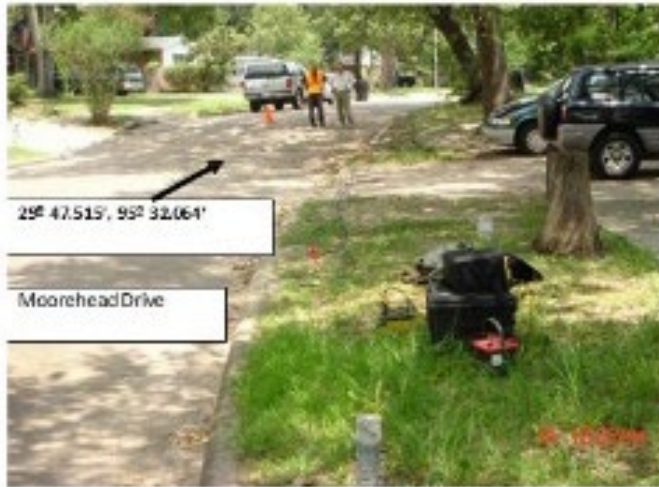
Figure 4. Picture showing coordinates of the Long Point fault scarp on the road and the location of resistivity profile. The view is to the north.
