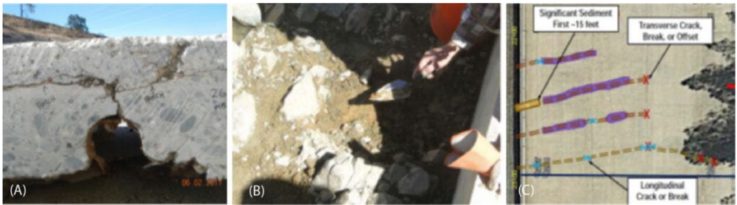
Figure 8. Results from destructive testing acquired during emergency response at the Main Spillway. (A) Thin concrete cover above a VCP drain in the vicinity of Station 26 (note lack of gravel filter blanket). (B) Sand and silt deposits above the bedrock surface in the vicinity of Station 26. (C) Results of video inspection of VCP drains at Station 22. From IFT (2018), Appendix D and Appendix I.
