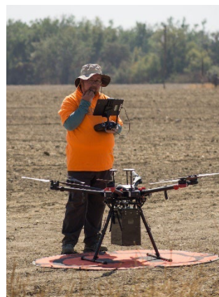
Figure: Preparing to test prototype payload for particle image velocimetry on the Sacramento River, California. Credit: Massimo Vespignani/NASA
