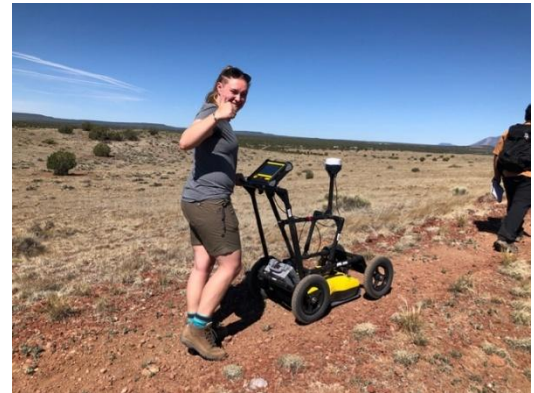
Student operates ground penetrating radar to image volcanic stratigraphy. Credit: L. Gallant
