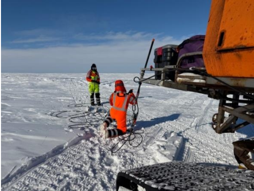
Crew setting up capacitive coupled resistivity survey in the Arctic. Credit: Esther Babcock
