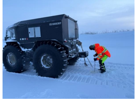
Measuring ice thickness to validate radar data. Credit: Esther Babcock
