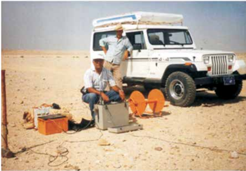
Figure 7: Equipment used for refraction seismic survey - 12 channel exploration seismograph (Geometrics model 1225).
