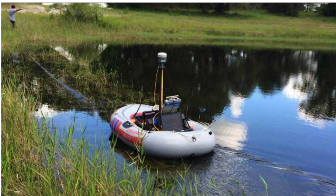
Figure 2: Floated GPR system; GPS antenna is installed at top of the GPR antenna.
