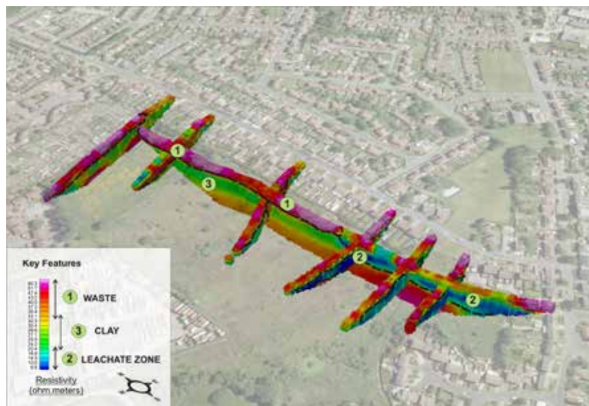
Figure 6: 3D view of the resistivity lines.
