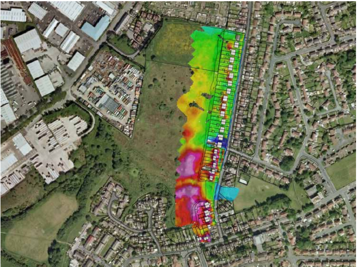
Figure 7: Conductivity data; red and pinks are high conductivity values (>50 mS/m), with green colours representing lower background conductivity.
