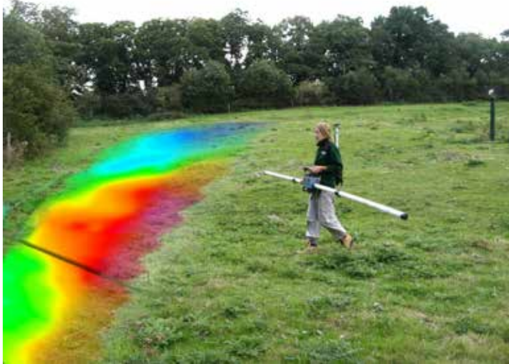
Figure 3: EM surveying with Geonics EM31 on a landfill. Schematic showing warm colors to denote presence of conductive waste mass.
