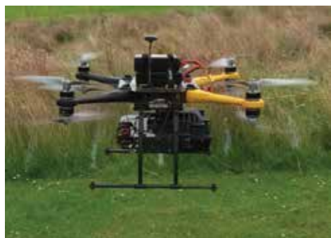
Figure 1: Ground Penetrating Rader by drone ( P. Deuck, et. al. – from presentation at PDAC 2017).
