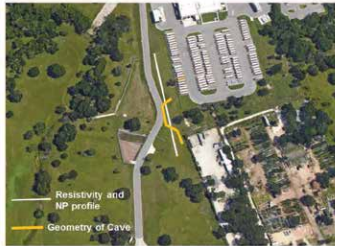
Figure 15: Site map showing the location of the geophysical profile, and the geometry of the cave, which was defined by trenching. The length of the geophysical profile is about 122 meter (400 feet).
