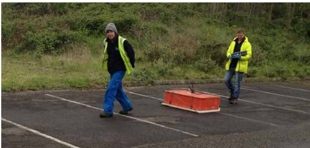
Figure 4: GPR survey with the 120MHz antenna.
