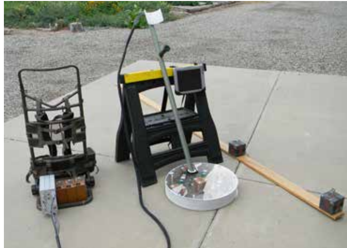
Figure 7: The MPV-II is a handheld time-domain EMI instrument that gives five three-dimensional data readings per sensor location. To the right of the sensor are the receivers from the MPV-II's beacon positioning system.
