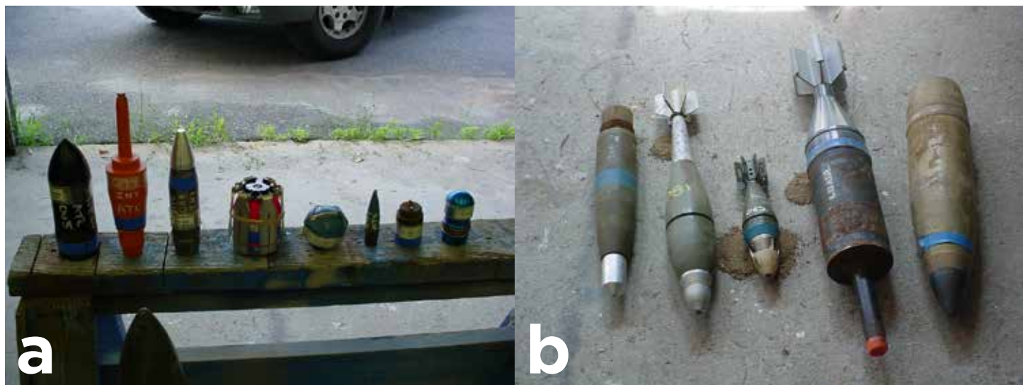
Figure 3: Ordnance items typically found in practice ranges in the United States. The UXO to be identified come in a wide range of sizes. Typical calibers range from 25 to 155 millimeters in diameter. a : 57-mm, MK-188 Rockeye, 40-mm, BDU and BLU bomblets, 25-mm, M42 grenade, and 40-mm grenade. b : 2.75" rocket, 81-mm, 60-mm, HEAT round, 105-mm howitzer shell.
