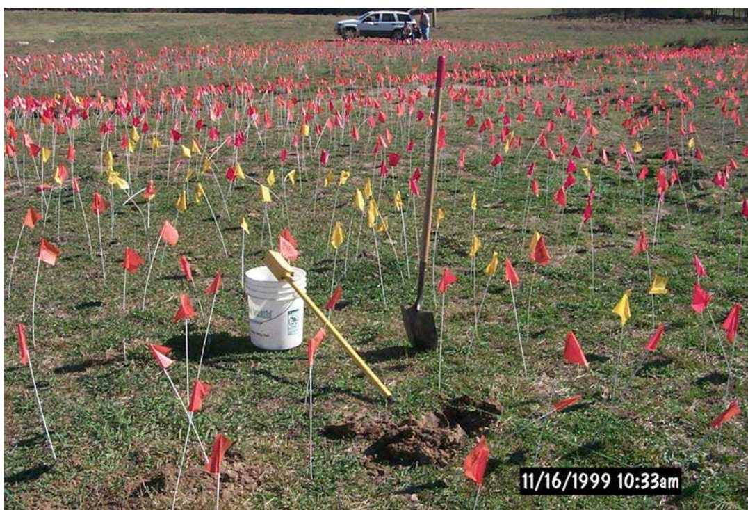
Figure 1: At the turn of the century, the search for UXO was carried out mostly with magnetometry, which can detect metal but cannot identify anything, resulting in an overwhelming number of false alarms. The magnetometer that took the data is leaning against the bucket in the foreground (photo courtesy of Roger Young).
