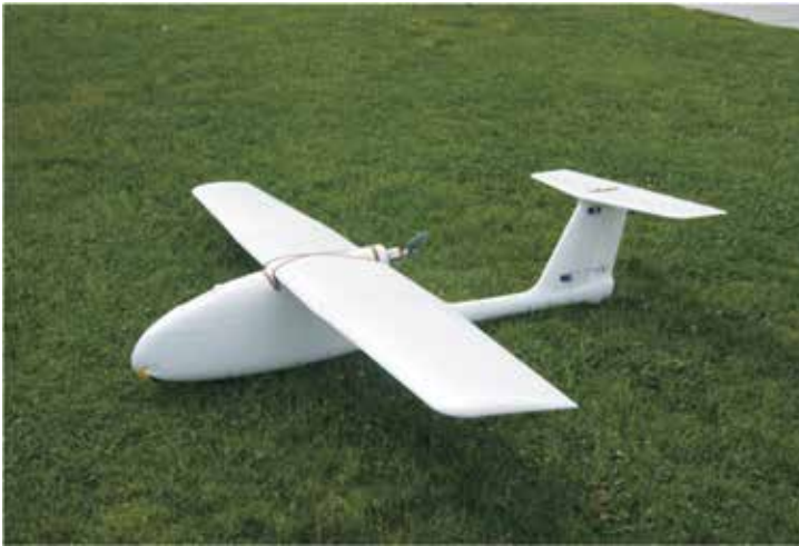
Figure 1: Hobbyist mapping UAS constructed of flexible EPO (Expanded Polyolefin).
