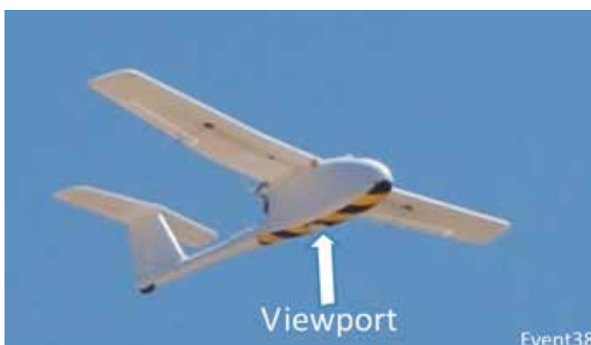
Figure 3: Fixed wing UAS with payload viewport.
