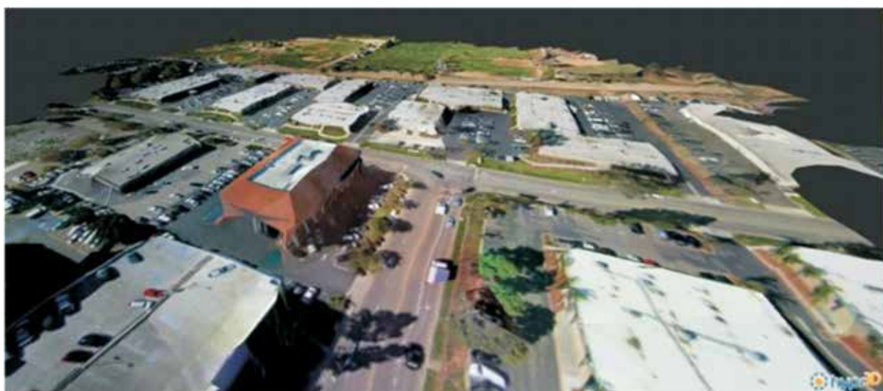
Figure 5: Near LiDAR quality imagery from hobbyist-grade UAS.
