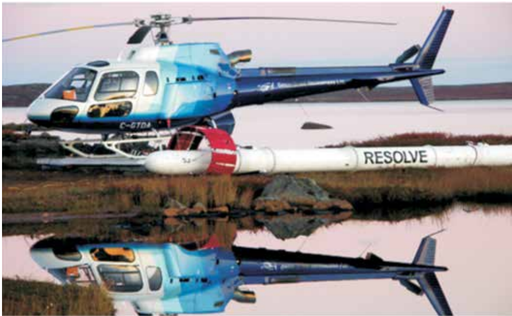
Figure 1: Multi-frequency RESOLVE® HEM System.
