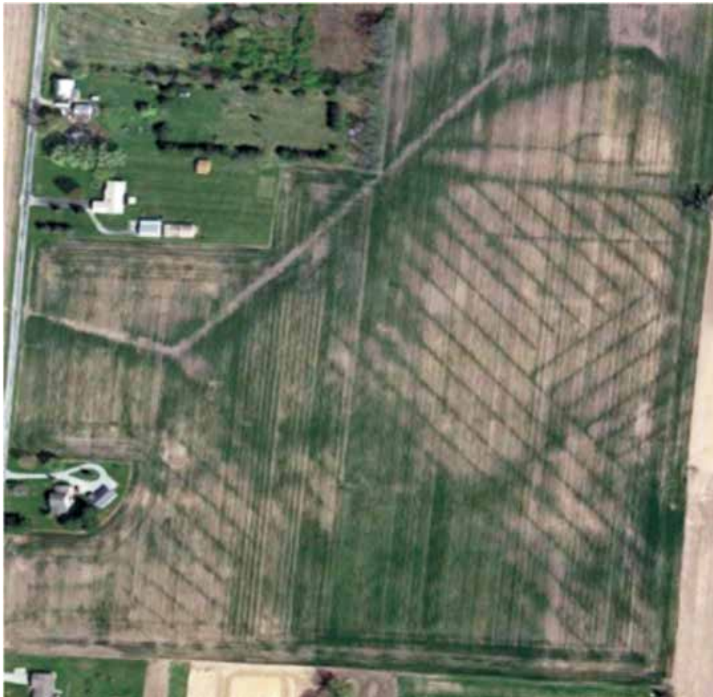
Figure 7: Google Earth image illustrating the dynamic effect of soil moisture and crop growth in revealing buried drainage tile network.
