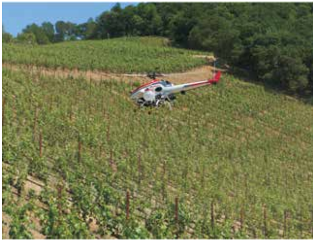
Figure 2: UAS spraying grapes, showing maneuverability and lifting power.
