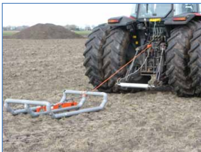
Figure 1. The gamma ray sensor the Mole in the lift of the tractor and the EM38 towed at the same time.
