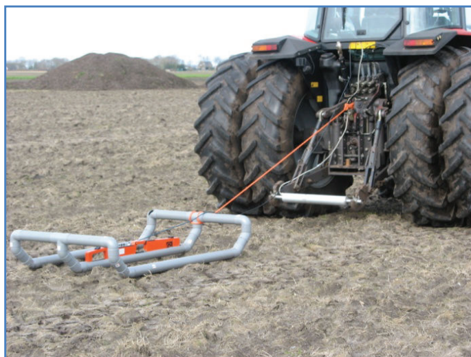
Figure 1. The gamma ray sensor the Mole in the lift of the tractor and the EM38 towed at the same time.
