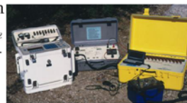
ZETA™ - Zonge Electrical Tomography Acquisition System
