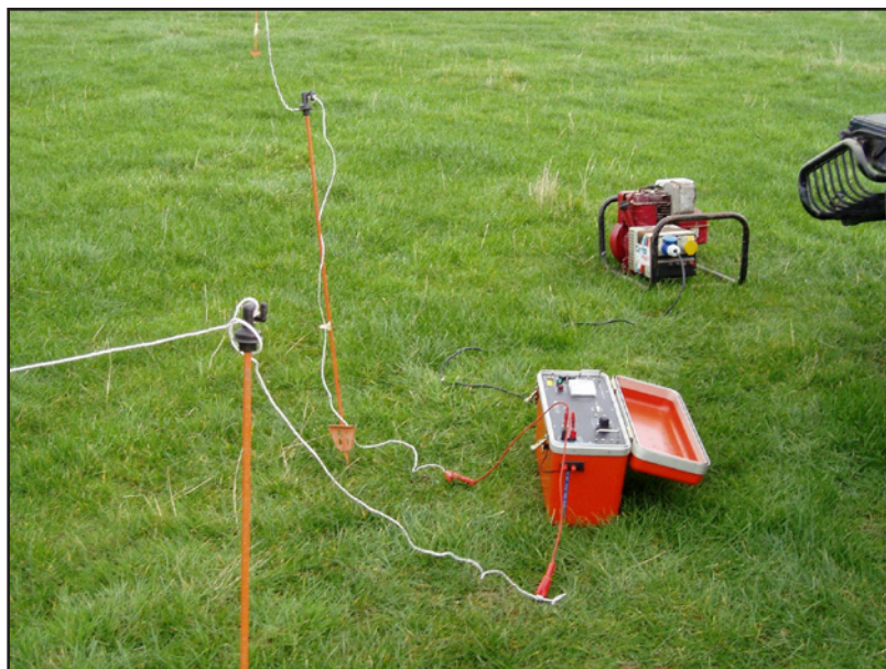
Figure 3. Tx27 (Geonics) portable transmitter with generator and wires leading to 1 km antenna.
