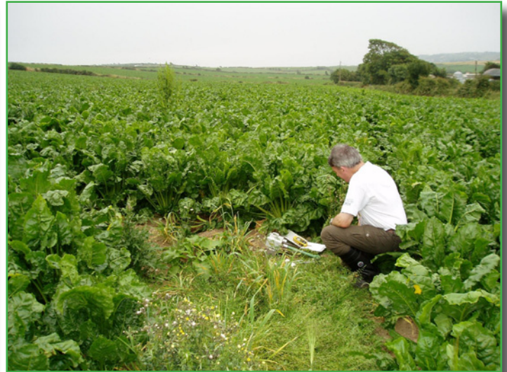
Figure 7. VLF-Resistivity in a cabbage field. Nick is doing the survey along the line of the drills so as not to damage the crop.
