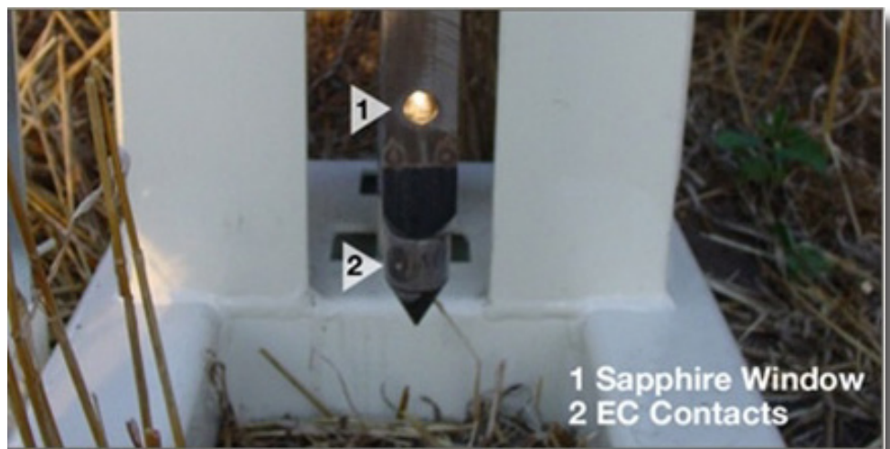
Figure 2: Probe window for Vis-NIR measurements and dipole EC cone tip.
