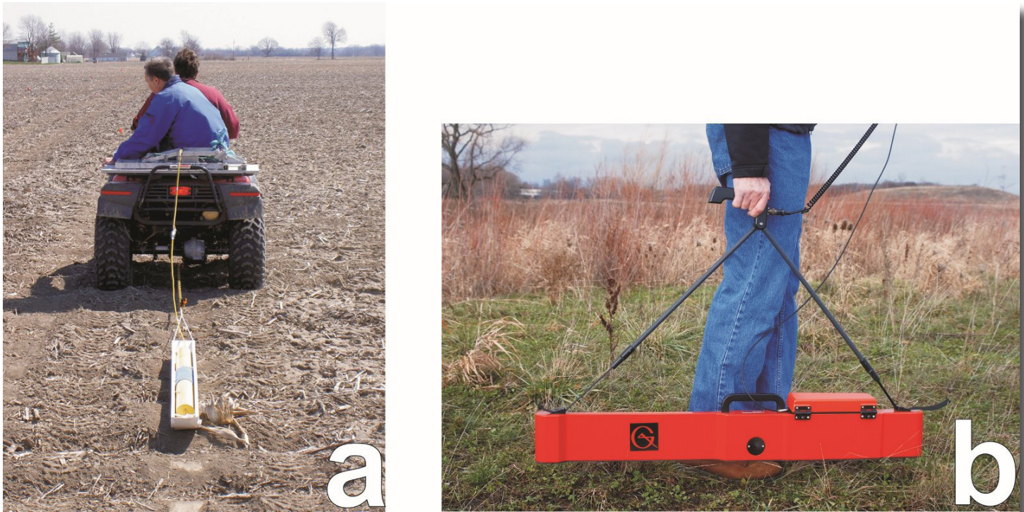
Figure 3. Examples of ground conductivity meters used in agroecosystem settings; (a) DUALEM-1S (Duaem Inc., Milton, Ontario, Canada), and (b) EM38-MK2 (Geonics Limited, Mississauga, Ontario, Canada).
