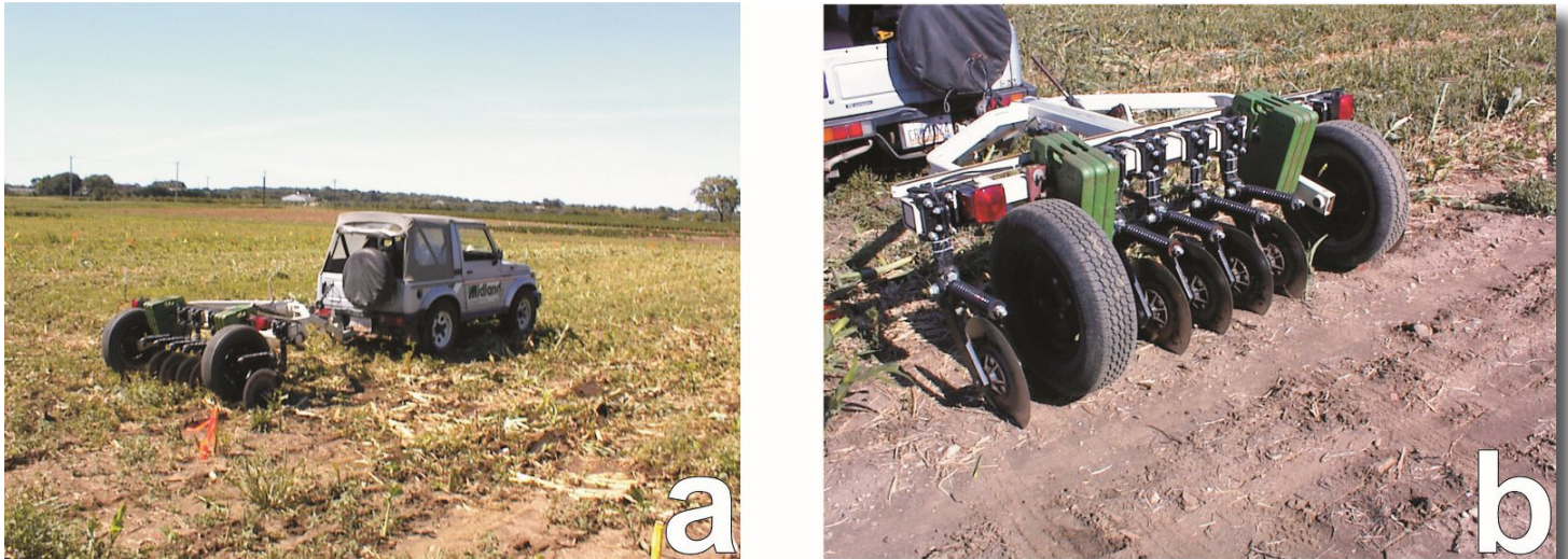
Figure 2. Example of a continuous measurement galvanic contact resistivity system; (a) Veris 3100 Soil EC Mapping System (Veris Technologies, Salina, Kansas, U.S.A.) and (b) close-up of steel coulters used for current and potential electrodes by the Veris 3100 Soil EC Mapping System.
