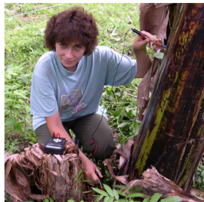
Figure 3: Correct placement of electrodes when measuring electrical potential difference between soils and plants with LandMapper ERM-02.
