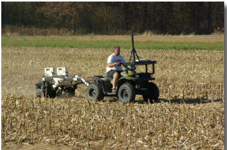
Figure 2. Soil EC_a sensing on an agricultural field has led to a better understanding of the spatially-variable soil health measures.
