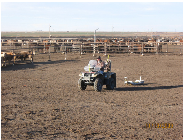
Figure 1. Electromagnetic induction system measuring the spatial manure accumulation on a feedlot surface.
