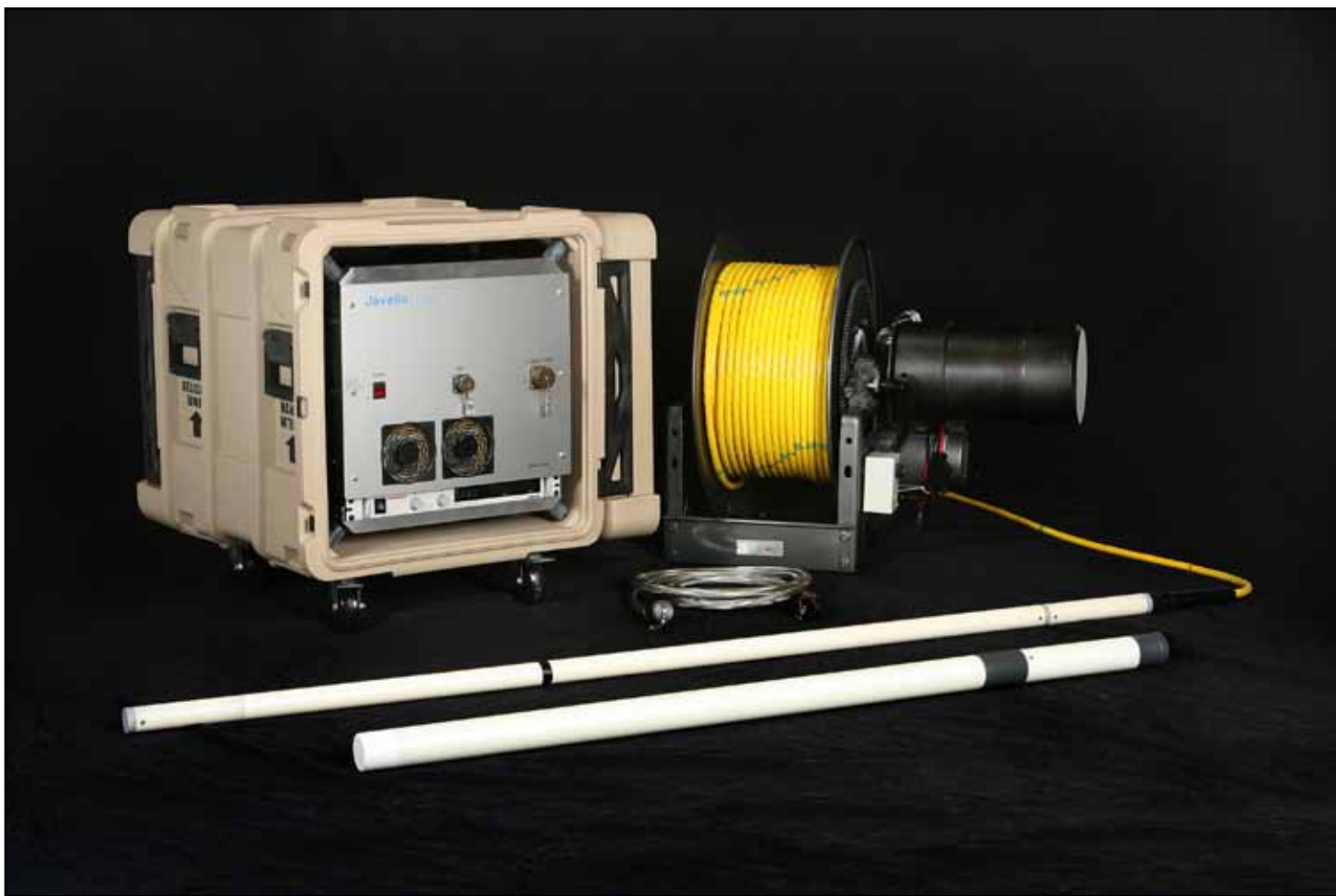
Figure 1: Javelin system components including rack-mounted surface electronics, cable winch with up to 600 feet of custom cable, and various connectorized downhole NMR probes. The 2.5" diameter Geoprobe® deployable probe and the 1.67" diameter borehole probes are shown in the foreground.
