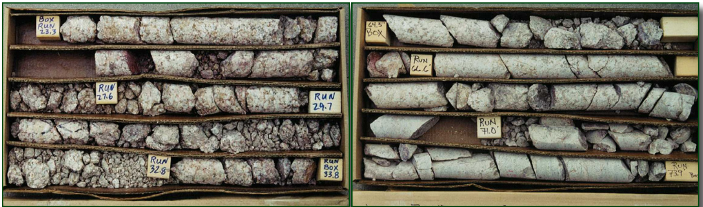
Figure 3. Examples of granite rock cores. The shallower, low RQD core on the left is from a zone with a seismic p-wave velocity of about 5,000 f/s (1,520 m/s). The deeper, higher RQD core on the right is from a zone with a seismic p-wave velocity of about 9,000 f/s (2,740 m/s).
