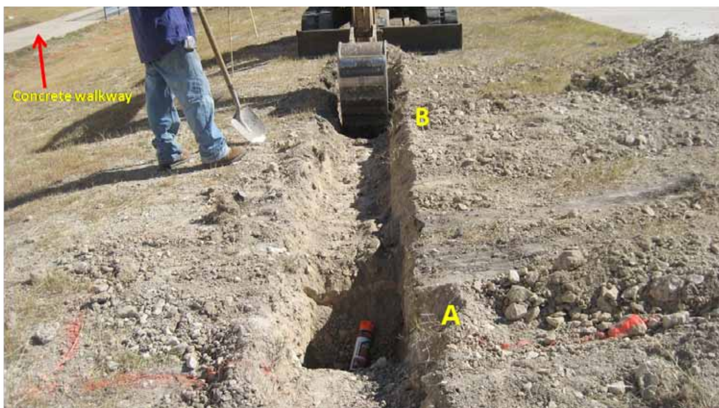
Figure 3. A trench showing the bedrock cuts A and B determined by the resistivity data. The rest of the bedrock cuts (C and D) was located later. The GPR data along this line did not show any anomalies. However, locations of these bedrock cuts were correlated well with the GPR data taken along the concrete walk way, which is located to the left.
