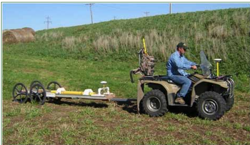
Figure 1. Subsurface sensor (Dualem 1-S) on trailer pulled by ATV using GPS to create maps.
