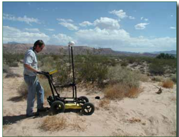
Figure 3. GPR has been successfully integrated with GPS in soil investigations.
