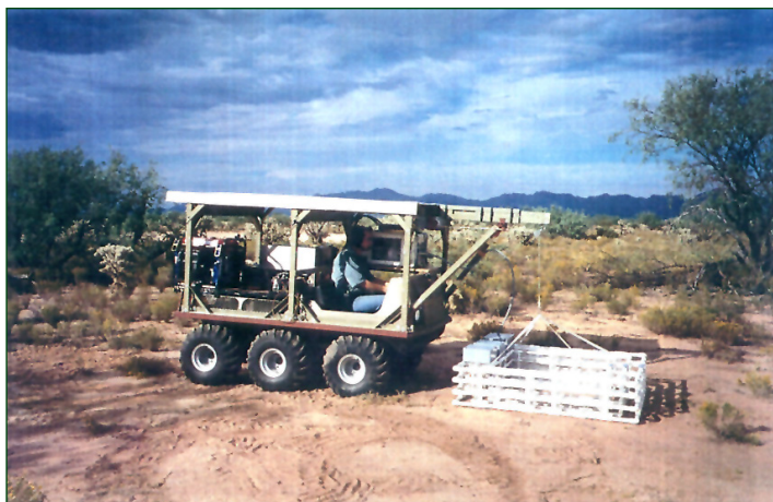
Figure 1. Photograph of the transmitter all-terrain vehicle with the transmitting antenna suspended from the boom in the front of the ATV.
