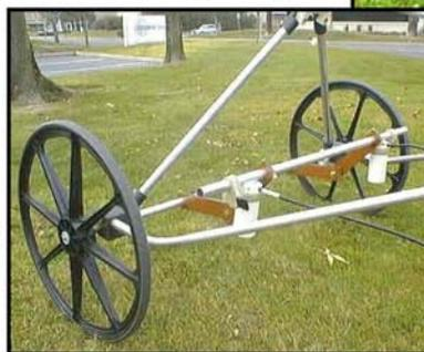
Left: dual sensor horizontal gradiometer
