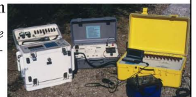
ZETA™ - Zonge Electrical Tomography Acquisition System
