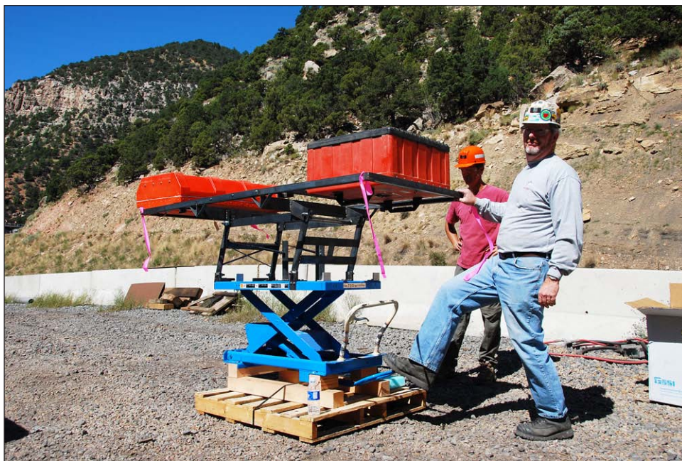
Figure 1. Custom-designed hoist apparatus for GSSI's 100- and 200-MHz antennas. The hoist, with elevation control, is mounted in the bed of a pickup for continuous radar profiling of the mine ceiling.
