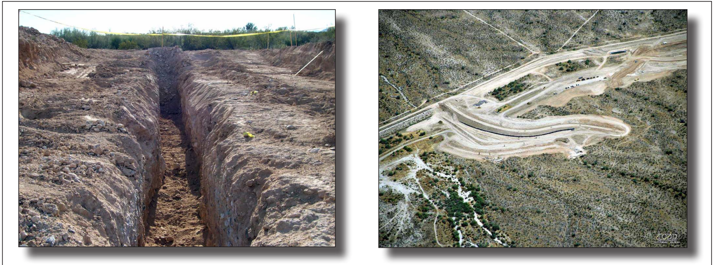
Figure 5. Test trench at new dam extension demonstrating various cementation conditions characterized with surface seismic (left) and final dam mitigation of extension that avoids earth fissure zone (right). At test trench, the upper horizon (p-wave velocities less than 300 m/s) has been stripped off to the top of a strongly cemented horizon (p-wave velocities 790 to 945 m/s) where backhoe refusal occurred. A larger trackhoe excavated through that horizon into the underlying less-cemented horizon (s-wave velocities 305 m/s). The final new dam extension is the curved section soil cement embankment at the center. The abandoned section in the earth fissure zone is to the upper right.
