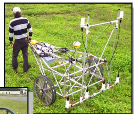
Above: six-sensor cart with concatenation box and GPS
