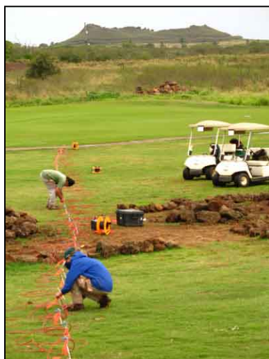
Figure 3. Supersting line setup across surface footprint of a lava tube on a golf course adjacent to the study site.
