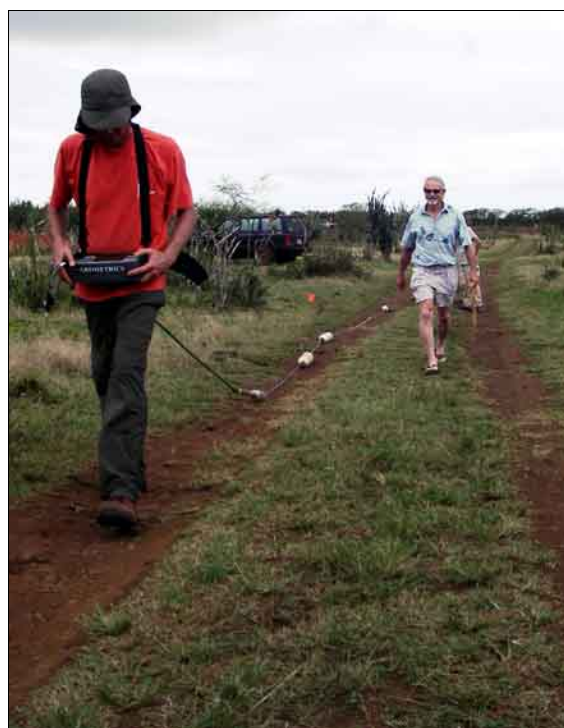
Figure 2. OhmMapper TR-2 (left) being towed by author. Cartoon (right) depicts dipole setup of the TR-2 system.
