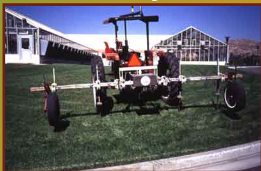
Four-electrode ER system
