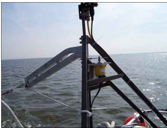
Figure 4. Tow point mechanism to allow tow cable angle measurement and provide GPS equipment mounting. The optical encoder and the tow cable weak link are visible.
