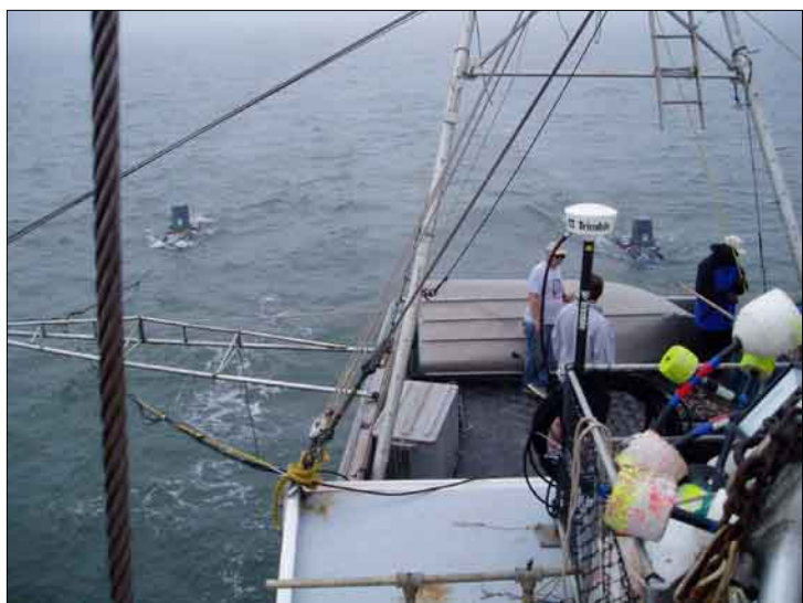
Figure 3. Sub-bottom profilers under tow, 12-m apart during the swath seismic/pseudo-3D field trial. The starboard outrigger can also be seen.
