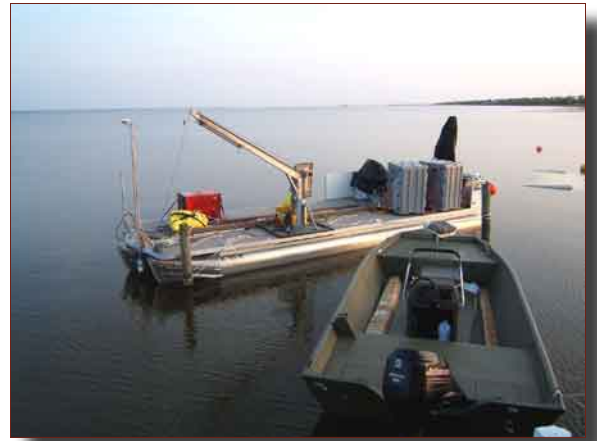
Figure 3. Triple float pontoon tow vessel outfitted with equipment for marine survey.
