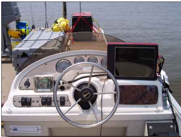
Figure 6. Navigational aids. The water depth indicator is immediately left of the steering wheel: The survey line display is to the right (and above) the steering wheel.
