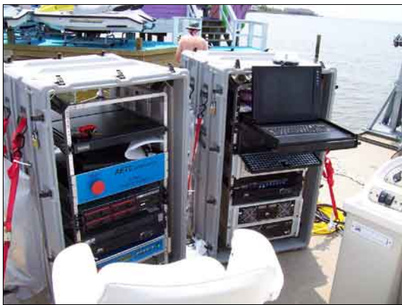
Figure 7. Instrument racks. Right rack: DAQ system with keyboard and LCD open. Left rack: SAIC DC power distribution unit (PDU).
