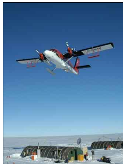
Figure 1. Aircraft over Thwaites Glacier field camp. Note radar antennas mounted below each wing.
