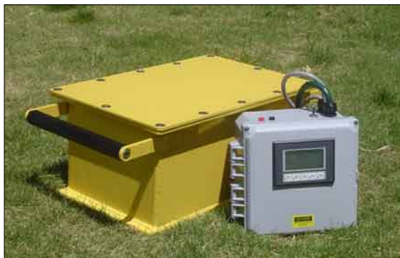
Figure 1. AutoSeis shear wave seismic source.
