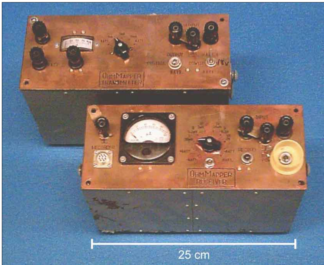
Figure 2. Analog transmitter and receiver of the North American prototype of the Russian-built VCHEP system as delivered to Geometrics. A second copy, shown here, came to the Geological Survey of Canada, and is still in good working order.
