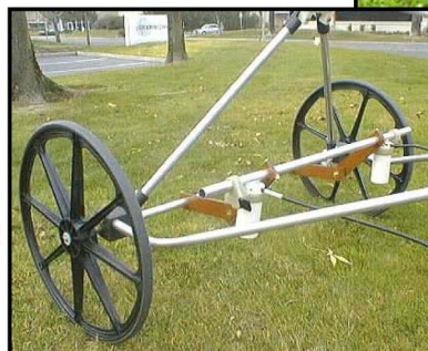
Above: six-sensor cart with concatenation box and GPS
