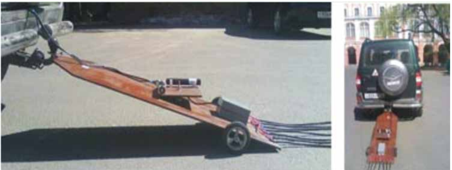
Figure 12. Measuring block formed by two horizontal magnetic antennae, electric signal preamplifier and electric antenna (Simakov et al., 2010).
