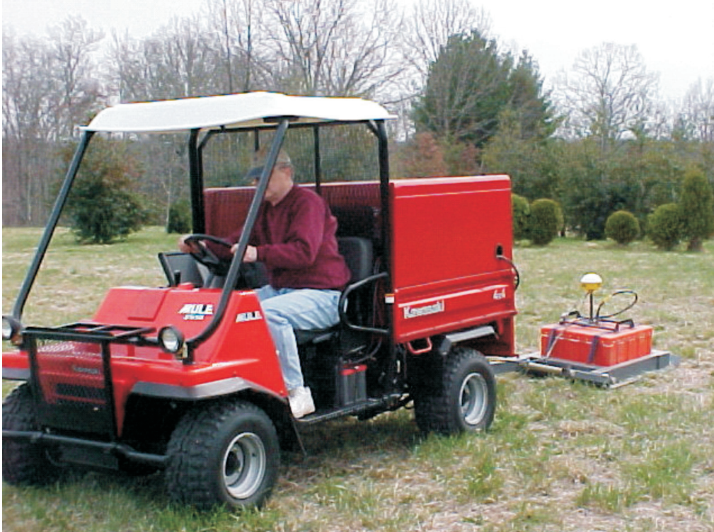
Figure 5: DGPS antenna mounted atop a shielded 200-MHz GPR antenna on sled.
