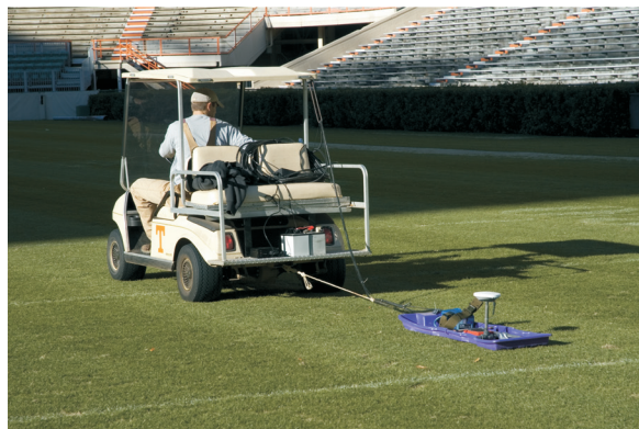
Figure 9: Surrounding aluminum bleachers in a collegiate football arena introduced significant GPS multipathing errors.
