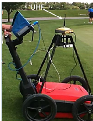
Figure 8: High-wattage UHF radio used to communicate with base station found to interfere with GPR.
