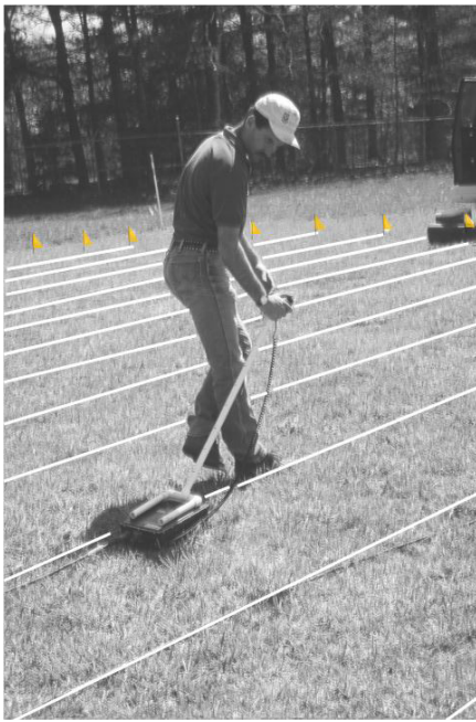
Figure 2: Grid survey layout, towed 900-MHz GPR antenna with hand switch.
