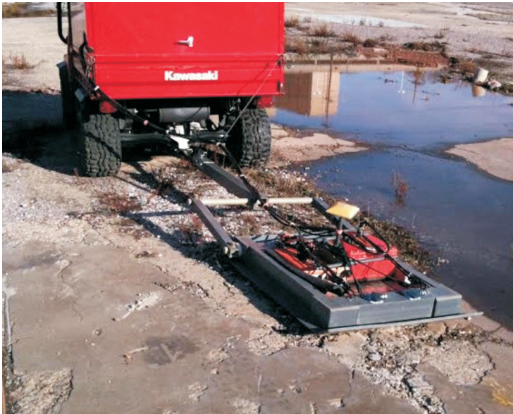
Figure 10: Dual GPR antenna array (400 MHz and 900 MHz, both shielded) with center-mounted RTK antenna on towed sled.
