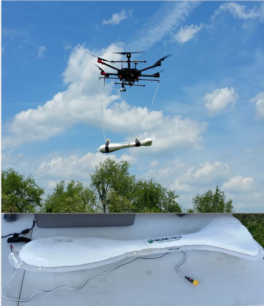
Figure 1: Geometrics MFAM Arrow prototype towed-bird used in early flight testing.
