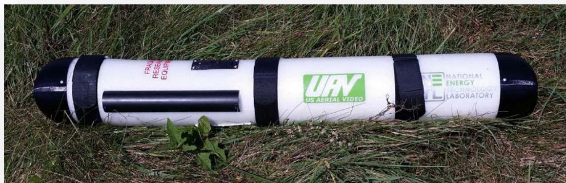
Figure 2: MFAM towed-bird prototype designed and built by NETL and US Aerial Video, Inc. used to locate legacy wells for the PATC.
