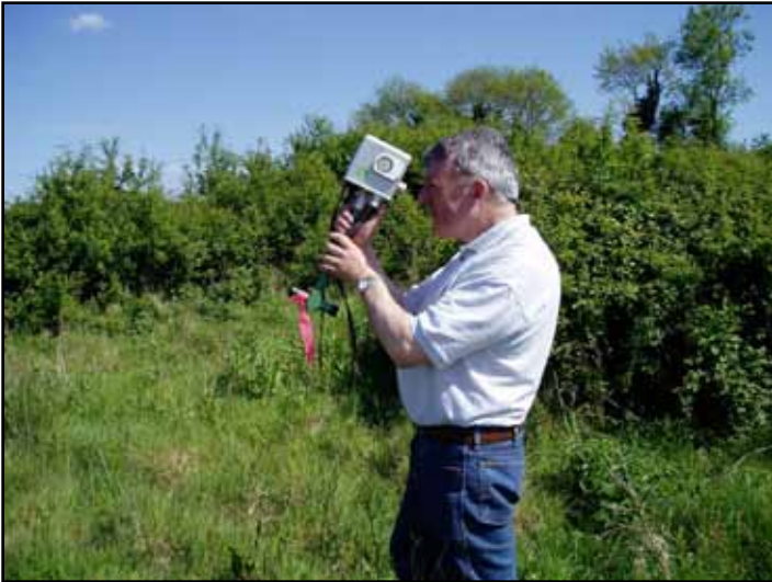
Figure 6. VLF-EM in Ireland. My colleague Nick is enjoying the fine weather. The upward tilt of the EM-16 signifies the presence of a conductive zone ahead of his position.
