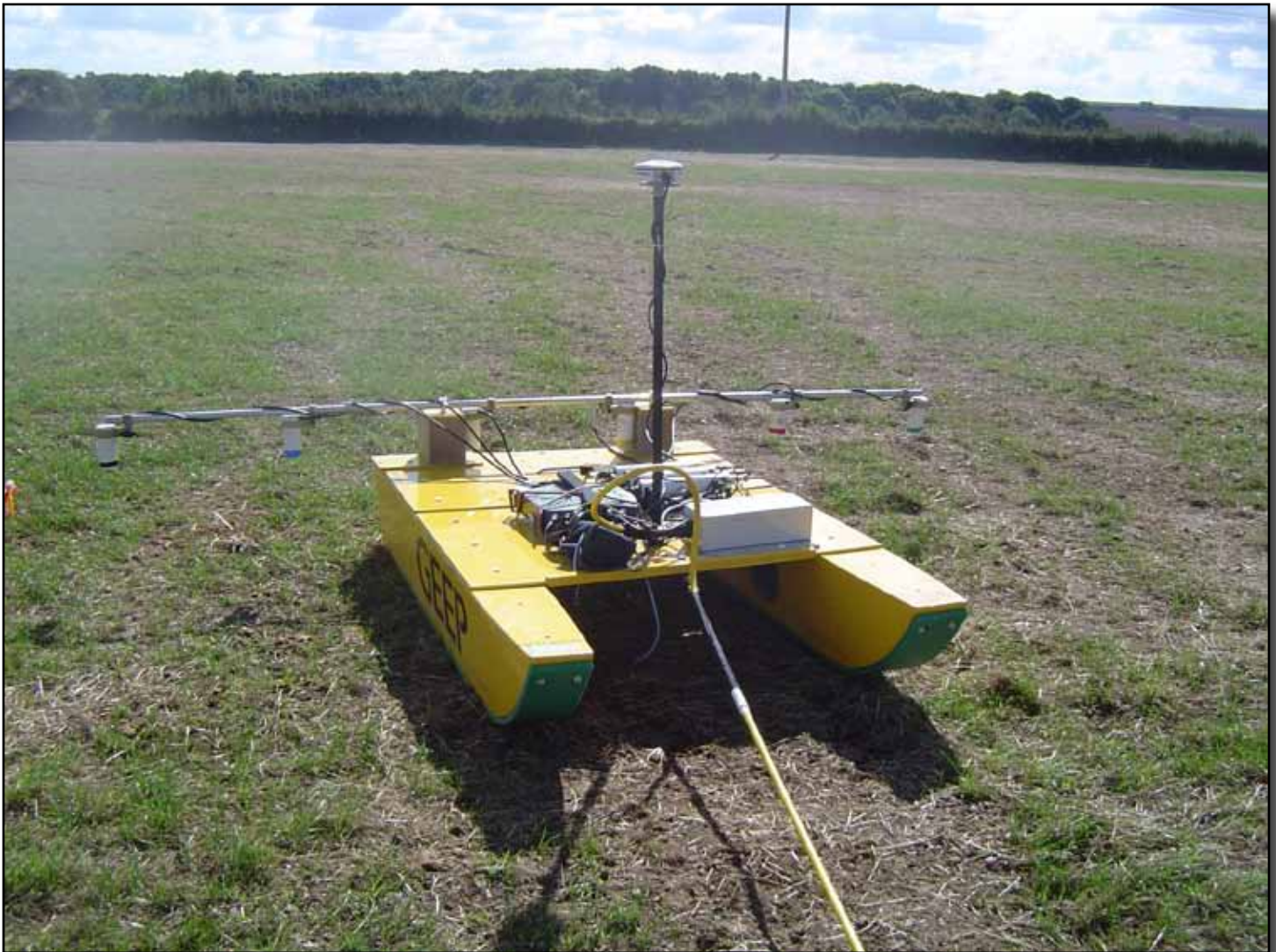
Figure 2. The GEEP (Geophysical Exploration Equipment Platform).
