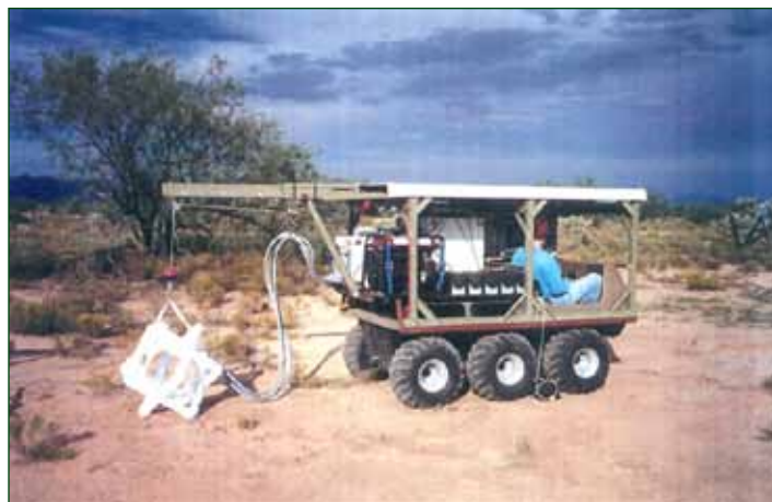
Figure 2. Photograph of the receiver all-terrain vehicle with the receiver antenna suspended from the boom projecting behind the ATV. In normal field operation this receiver ATV leads and the transmitter ATV follows along the profile line.
