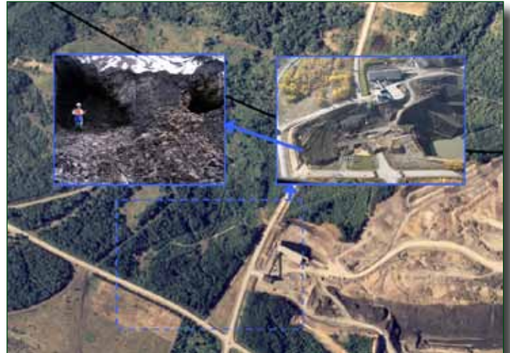
Figure 1. Aerial photograph of the Stellerton Mine expansion block before mining (dashed box), after the start of mining in Fall 2005 (inset, upper right) and openings mapped in the pit end face (inset, upper left).
