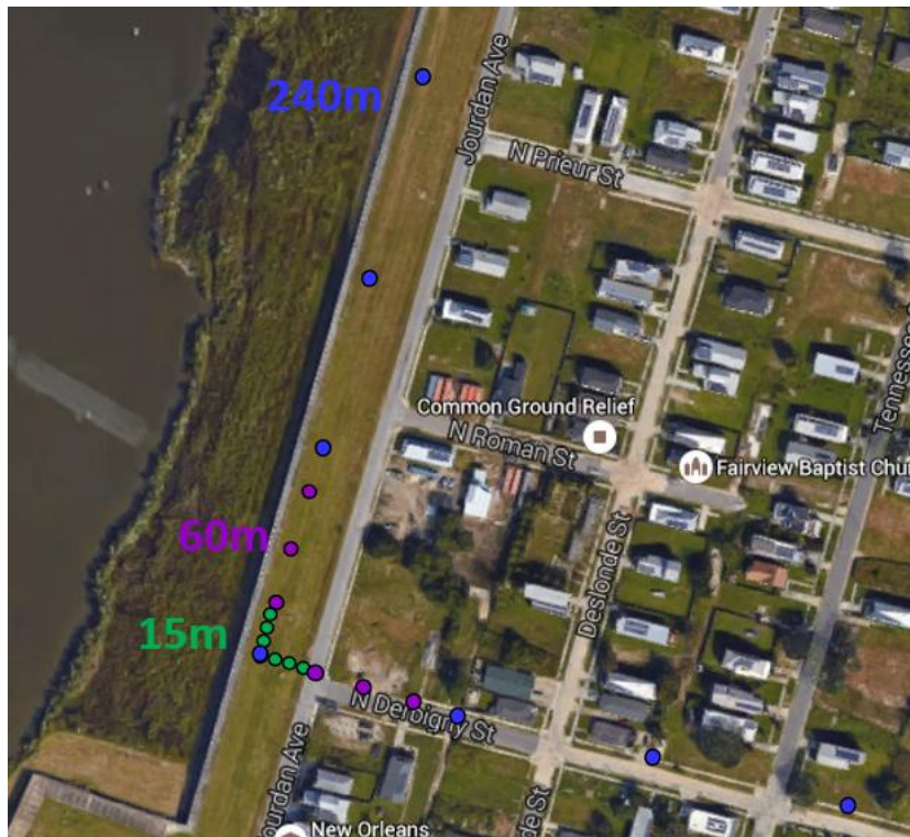
Figure 7: Configuration of L-shaped arrays for 1D deep investigation at the Industrial Canal.
